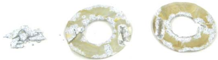
Figure 3: Aluminum fins from a geothermal power plant subjected to 24,000 cycles of exposure to briny conditions with: no protective coating (left), nano-coating with a low level of Cerium Oxide (middle), and a nano coating with a higher concentration of Cerium Oxide (right).
