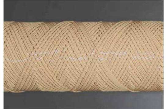
Figure 2: PEEK Hollow fiber membrane contactor developed to increase the efficiency of carbon capture from power plant flue gas
