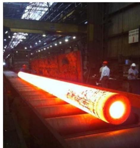
Figure 1: Extrusion of Inconel 740H Pipe at Wyman Gordon plant
