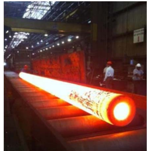
Figure 1: Extrusion of Inconel 740H Pipe at Wyman Gordon plant
